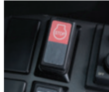
Emergency stop switch
