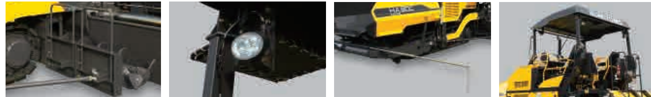
Screw guard Rear LED auxiliary lighting Traveling indicators Hard top (FRP) canopy
